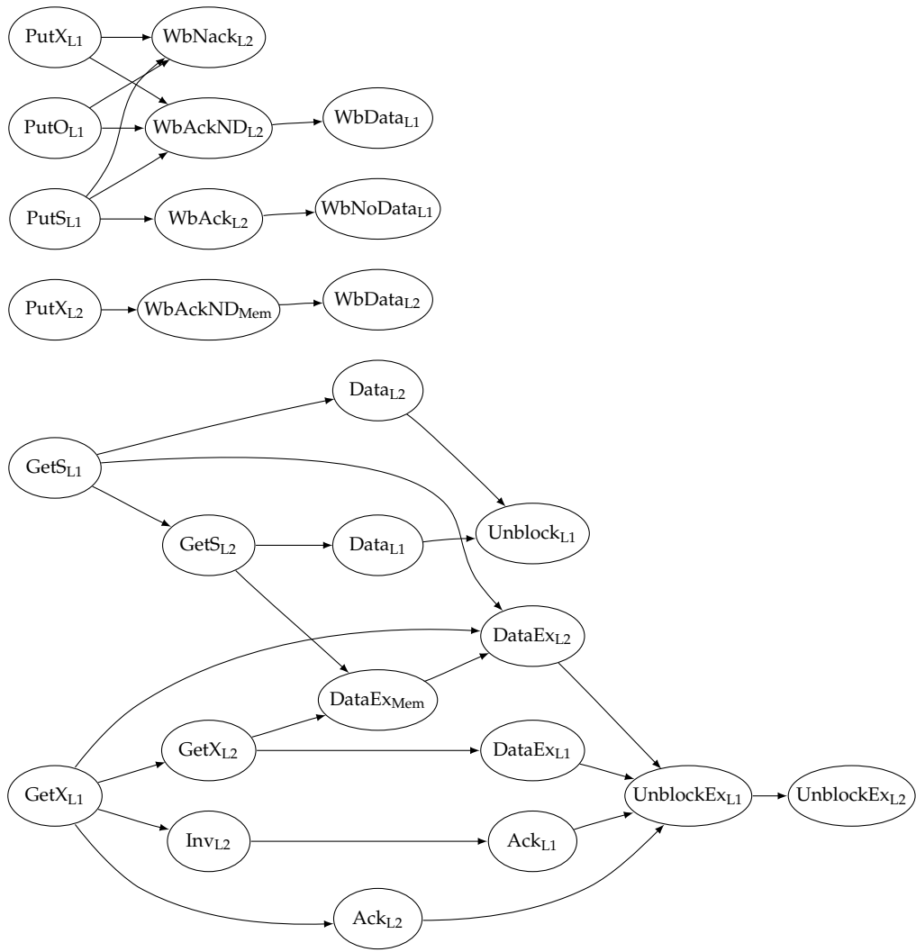
Figure C.1: Message dependency chains for the DIRCMP protocol
