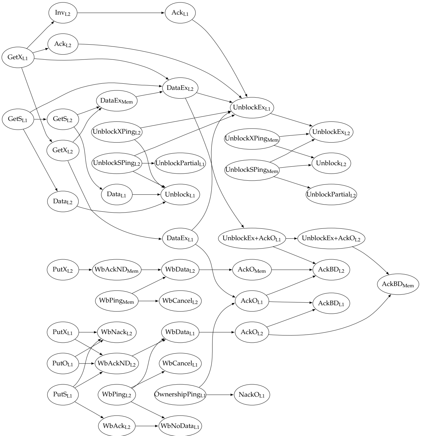
Figure C.2: Message dependency chains for the FTDIRCMP protocol
